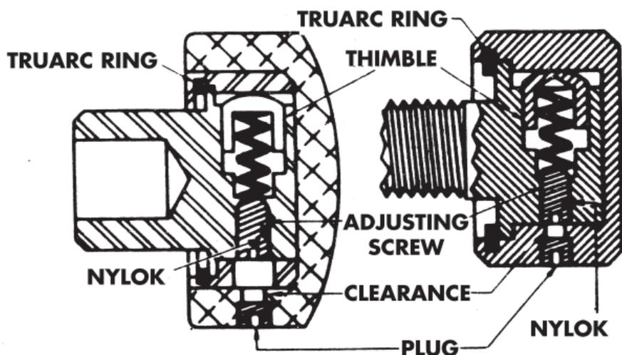
It is not necessary to disassemble the Vlier Adjustable Torque Thumb Screw or Torque Handle to adjust the end pressure. Adjustment is made through the head, as follows:
